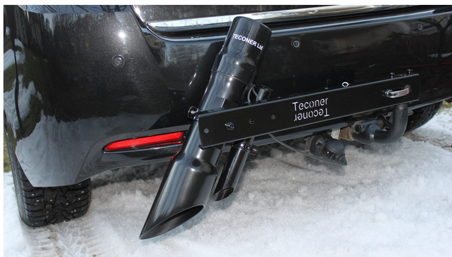
Figure 4.1: A Teconer RCM411 sensor system [27] attached to a car (image source https://www.teconer.fi/en/surface-condition-friction-measurements/#RCM411 ).
